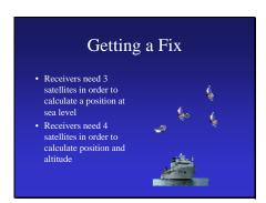
In the three dimensional world, it takes four spheres, rather than three circles, to determine your position. A receiver can calculate your position at sea level with three satellites (Three spheres plus the earth as the fourth sphere). Four satellites are required to calculate position and altitude.
